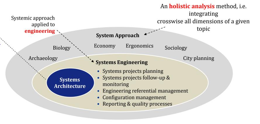
The respective perimeters of systems engineering & systems architecture inside the global perimeter of system approach
